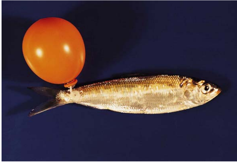
Figure 1. HI-Z Turb N' Tag attached to a juvenile American shad. After passage through a hydraulic control structure, the tag inflates (as shown) and buoys the fish to the surface for recapture by a boat crew.
